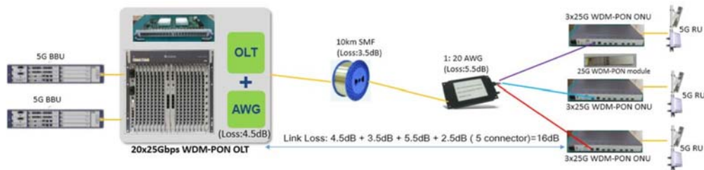
Figure 4.18 Experimental setup of a real-time WDM-PON system for 5G front-haul supporting 20 pairs of bi-directional 25-Gb/s signals [7].
