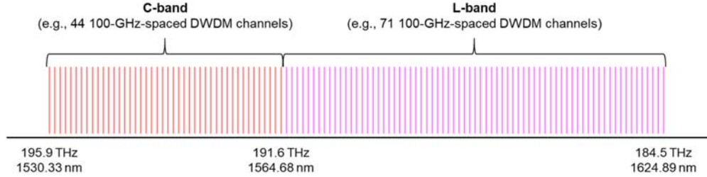
Figure 4.7 The ITU DWDM channel plans in the C-band and the L-band.
