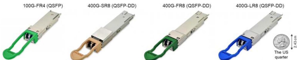
Figure 7.14 Pictures of representative color-coded pluggable format factors used in intra-data center connections.
