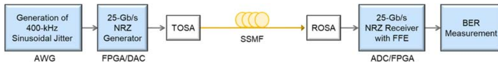
Figure 10.14 Experimental setup for the jitter tolerance study. After Liu X, Shen A, Cheng N, Jitter tolerance mask for 50G-PON . In: Contribution D12, ITU-T SG15/Q2 Meeting; February 2021 [38].
